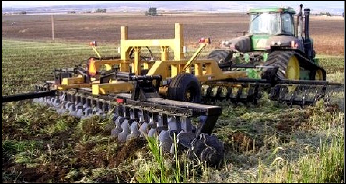
Rome Model 4250-53-WF Wheel -Type Offset Disk Harrow Plowing Stubble.
